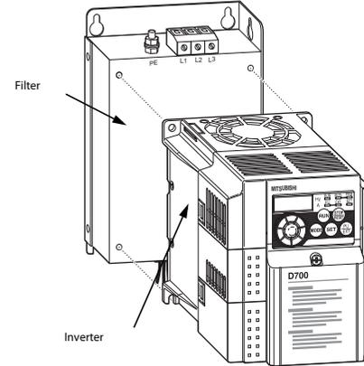
To fix the filter-inverter unit on the cabinet back panel use proper screws (not provided with the filter). For correct filter performance the filter should electrically bond to the cabinet back panel which needs to have proper connection to earth. If needed please remove the paint under the filter footprint.
